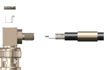
2) Insert the cable into the body, ensuring that the cable braid is on the outside of the connector mandril and that the centre core locates in the internal mounting post
