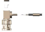
2) Insert the cable into the body, ensuring that the cable braid is on the outside of the connector mandril and that the centre core locates in the internal mounting post
